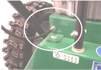
Blade Cable Adjustment
